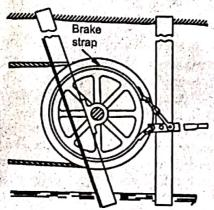
Fig. 15.11 Jig pulley of gravity haulage
