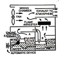
Fig. 16.7. Exhaust conditioner and flame trap used in u/g diesel locos
