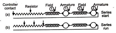
Fig. 16.10. Different electrical connections in a series wound D. C. motor of an electric trolley or battery loco having two motors.
