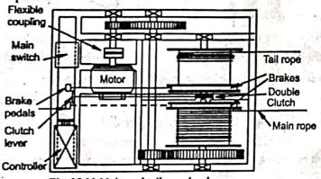
Fig. 15.10 Main and tail rope haulage
