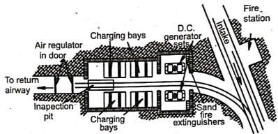
Fig. 16.8. Battery charging room layout.
