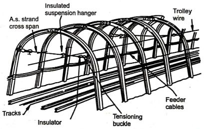
Fig. 16.9. Trolley wire for trolley wire loco.
