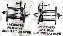
Fig. 8.5 Winding on drum
