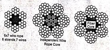
Fig. 8.1 A cross-section of round strand ropes.
